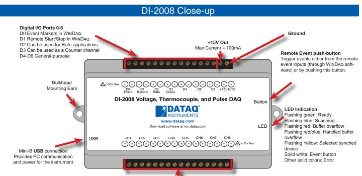
Analog In Channels 1-8 (programmable Voltage or Thermocouple) Voltage Ranges: ±10, 25, 50, 100, 250, 500 mV; ±1, 2.5, 5, 10, 25, 50 V; Thermocouple Types: J, K, T, B, R, S, E, N
