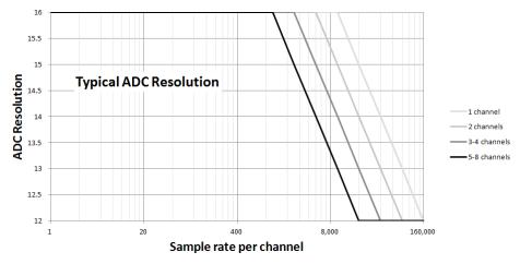
ADC resolution (R) is a function of selected sample rate per channel (F), and the number of enabled analog channels (C):
