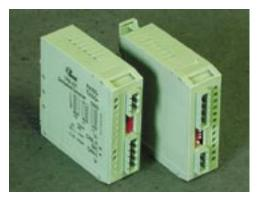
The 1782-JDC is a family of DeviceNet-to-serial link communications gateways that provide a flexible DeviceNet interface to a wide variety of ASCII devices. The JDC allows the user to easily and conveniently connect and integrate peripheral products with either RS232 or RS485 serial ports into a DeviceNet system.
